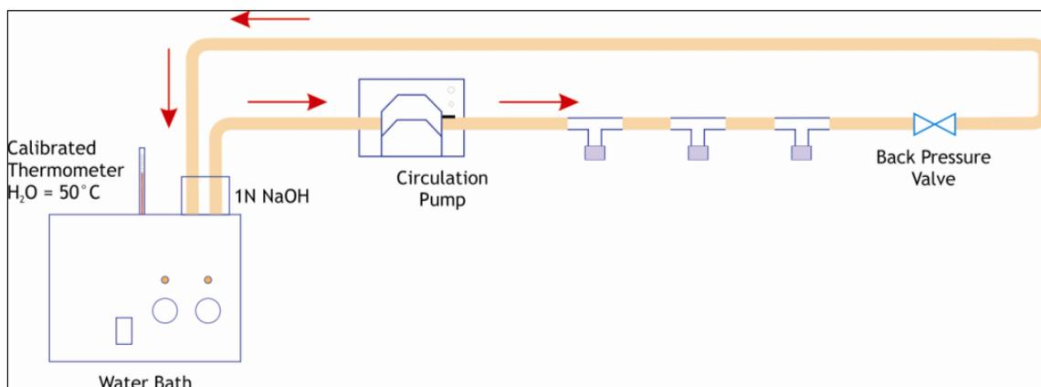
Flow rate was set at 340 ml/min with size 16 tubing in the pump head and transitioned to 3/8" ID tubing with a plastic reducer fitting. Pressure in the system was <5 psi. Caustic flow was
