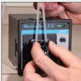
2. Insert tubing in right or left retainer and wrap tubing around the rollers. Secure tubing in opposite retainer.
